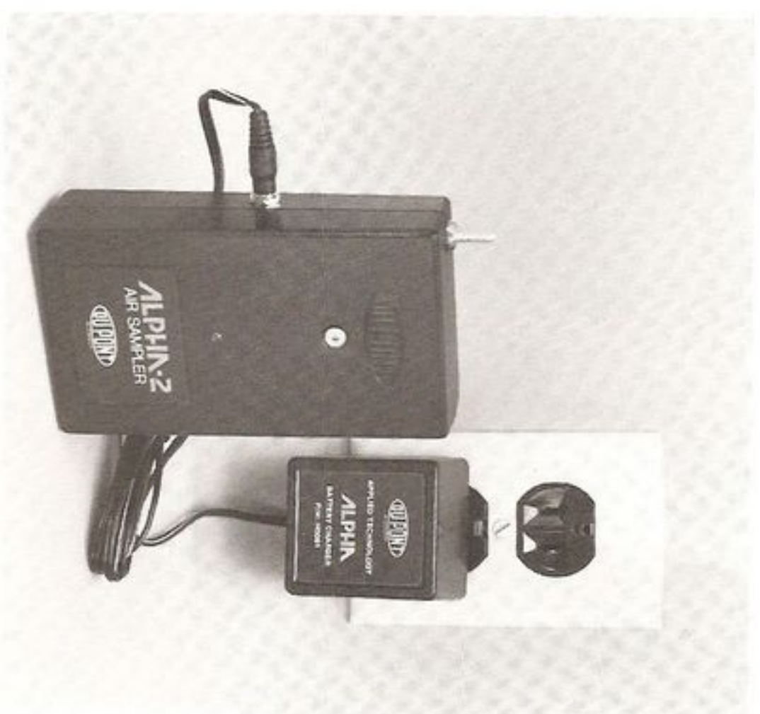
Figure 9. Battery Charger in Use.
