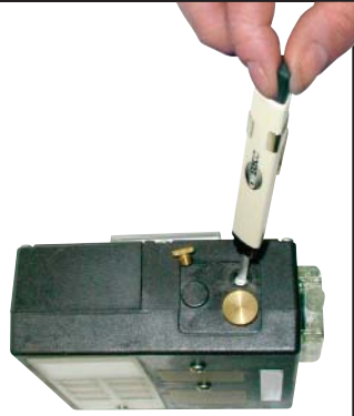
For low flow, turn valve screw counterclockwise.
